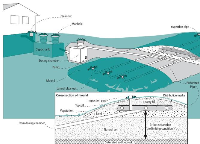
Figure 1. Cross section of a mound system.
